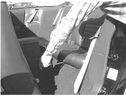
Remove the back seat
