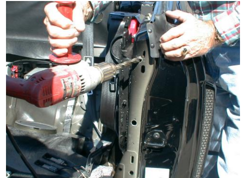
Drill two holes at 3/4" to B-pillar
