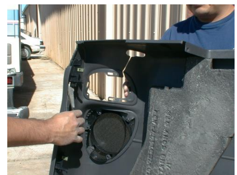
Remove plastic brackets
