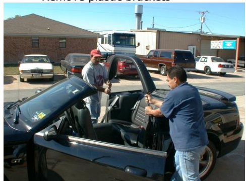
Install bar with two people pushing against each other
