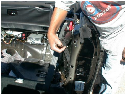
Place bracket BEHIND the B-pillar
