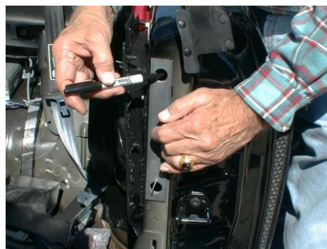
Insert small rivet, mark the holes at B-pillar
