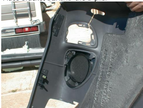
Make openings at top of panel
